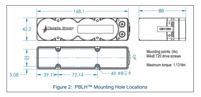
Dimensional spacing of the mounting holes for the modules is shown in Figure 2.
